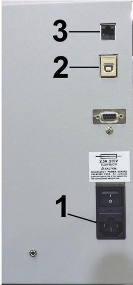
2. Plug the power cord into the receptacle [1] located below the main power switch. The internal power supply in the printer is rated 100 to 240VAC, 50/60 Hz.
