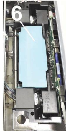
**Note:** When priming stops, open the top cover and check that ink is flowing through the hoses. If air bubbles appear, tap the lines and close the top cover. Or close the top cover and click **Circulate Ink** on the touchscreen to clear the air bubbles.
